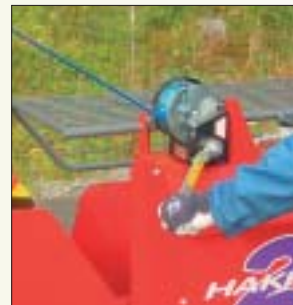
The conveyor height is adjusted with a hand operated self-locking winch.
