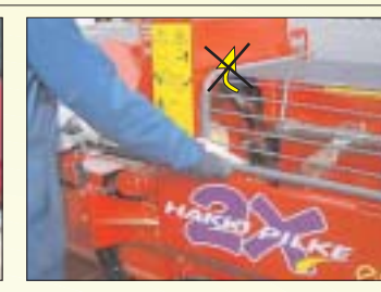
Emergency stop and splitter reverse. The splitting chamber guard cannot be opened while splitting is in progress.
