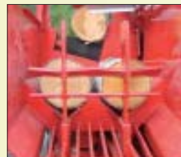
A 6 way splitting blade is available. The 63 mm cylinder is recommended.
