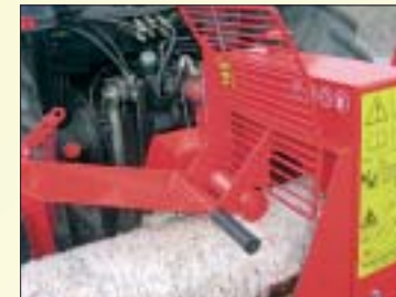
The spring-loaded support roller automatically opens the guard.
