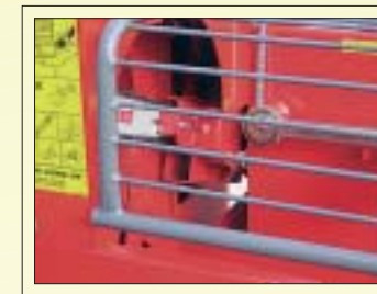
When the guard for the splitting chambers is open the cross cutting saw is locked.
