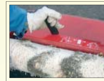
When the guard for the splitting chambers is open the cross cutting saw is locked.
