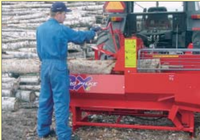
Transfer and cross-cutting of the wood by hand.
