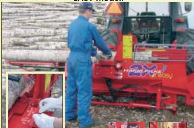
The feed conveyor carries the log into the machine. Machine operation is by the hand lever. EASY model:
