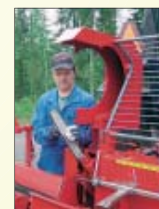
After one securing bolt is removed the sawbar cover can be fully opened to allow easy access for maintenance.
