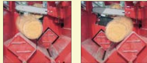
The wood is automatically guided into the vacant splitting chamber.
