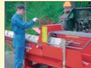
Ergonomically correct working position. The cutting and splitting areas are fully guarded.
