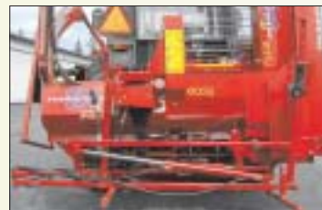
The hydraulic log lifter folds behind the machine for transport.
