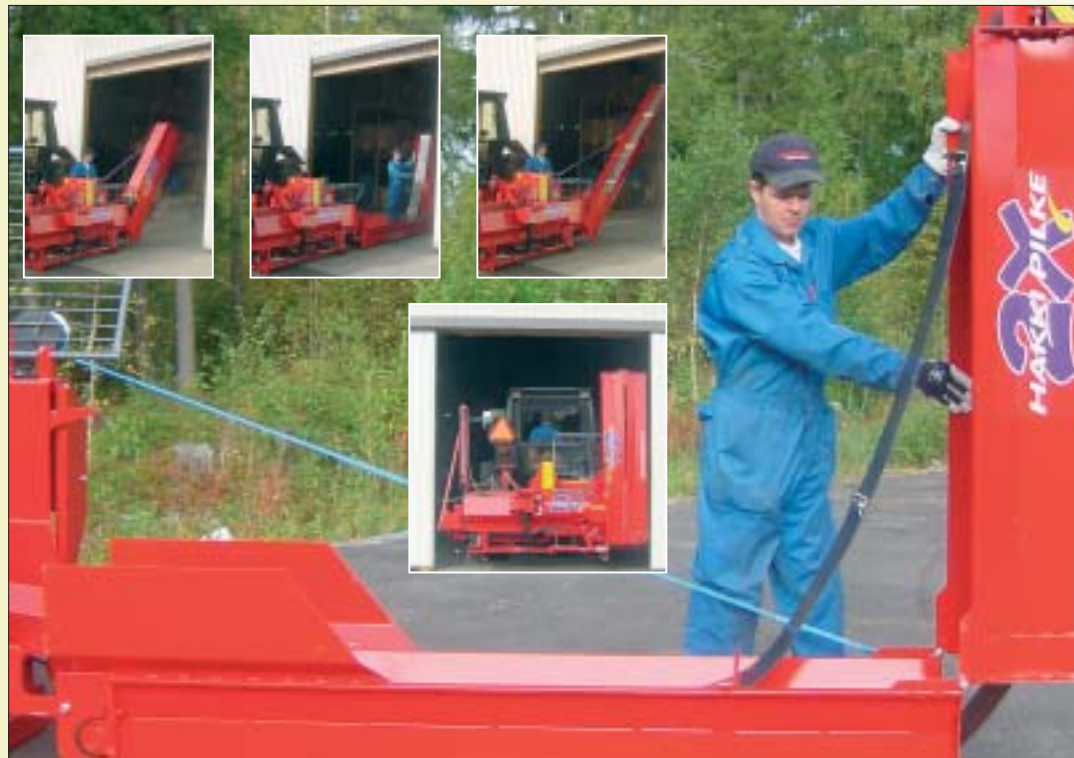
The conveyor height is adjusted with a hand operated self-locking winch.
