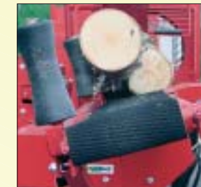
The slightly inclined infeed conveyor keeps the logs safely on the table.
