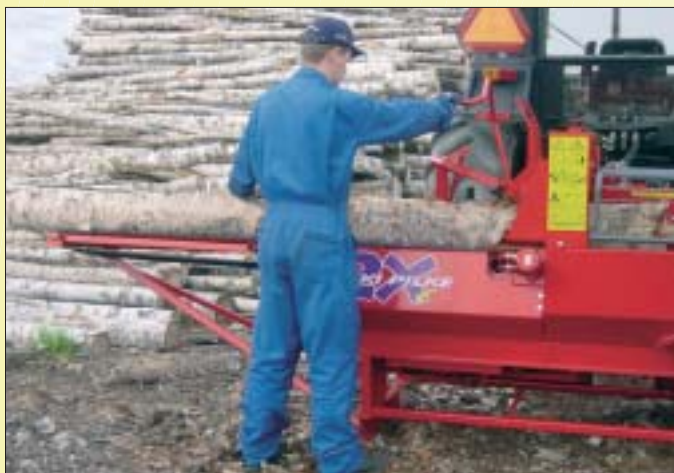
The feed conveyor carries the log into the machine. Machine operation is by the hand lever. EASY model:
