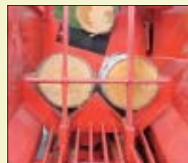
With the standard blade wood can be split into 2 or 4 pieces.
