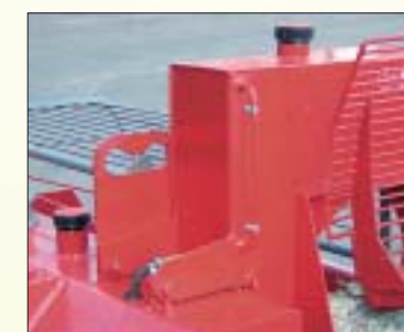
Automatic chain lubrication! Oil goes to the chain only when the machine is in use. There are separate tanks for hydraulic oil and chain oil.
